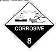
UN 1719 CAUSTIC ALKALI LIQUID N.O.S. (SODIUM HYDROXIDE) CLASS 8 HAZCHEM 2R PG II
